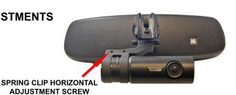
3 - Using the upper and lower pivot screws, adjust the mount to achieve your desired location of the dashcam. We recommend adjusting it as high as you can. You can also use the spring clip horizontal adjustment screw to help center the dashcam with the mirror as shown above.
